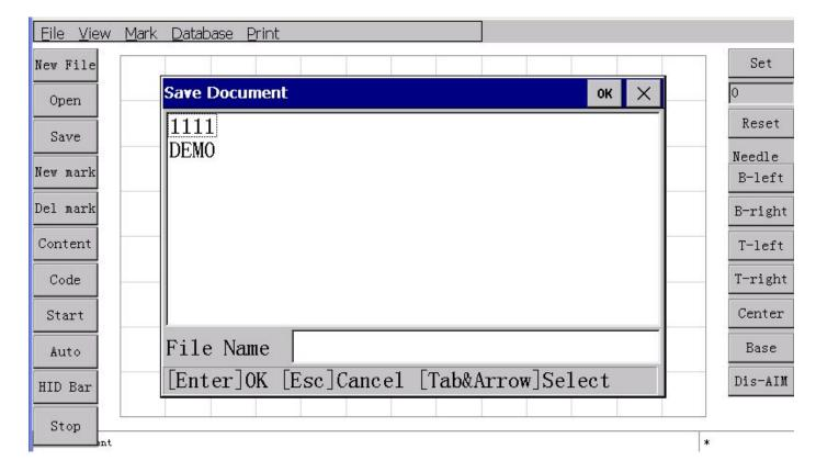
"Save" Window lists all the files in the development of engraving machine, enter a file name in the "file name" column, and then click the top right corner of the window (OK) button or press (Enter) key, the file is saved.
