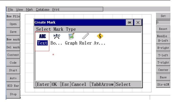
Here we select "mark text" type, and then click the top right corner of the window (OK) button, or directly press the Enter key, finish marking type selection. Then "edit the markup content" window opens automatically, as shown in the following
