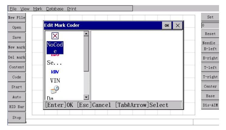
Because we want to make the tag content for fixed content, which means they do not need to change in the imprint is finished, so here we will use the default "no code". Click again on the top right corner of the window (OK) button, appeared engraving engraving control software operating area in the tag we established, as shown below:
